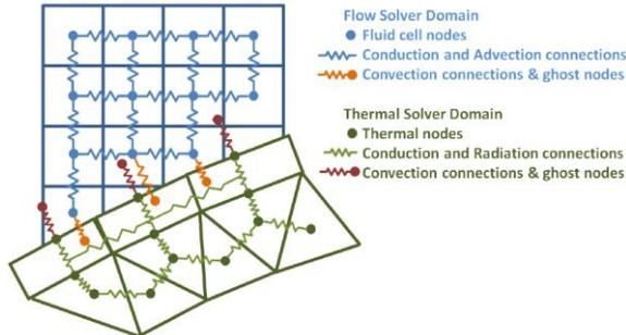
Figure 1: Domains of the flow and thermal solvers.
