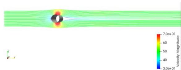
**Figure 8:** Conventional CFD results for cylinder in crossflow (computed heat rate = 637.4 W)
