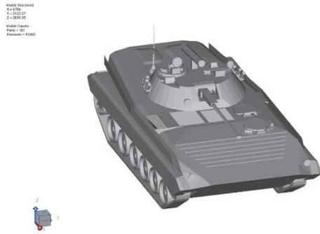
Figure 3: Thermal model geometry for BMP-2
