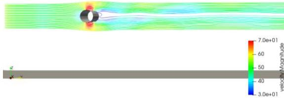
**Figure 9:** RapidFlow results for cylinder in crossflow (computed heat rate = 611.3 W)
