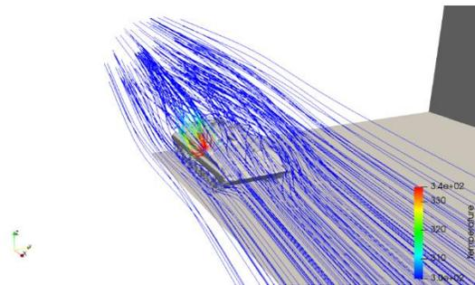
Figure 4: RapidFlow simulation streamlines colored by temperature, BMP-2 model, exercised
