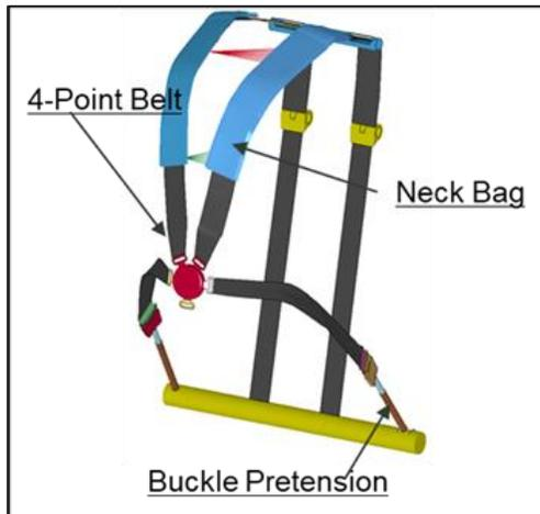
**Figure 7:** 4-point seat belt with neck airbag
