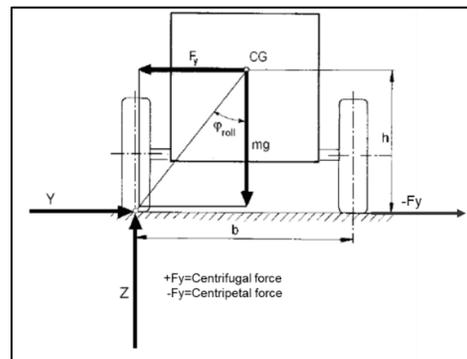
**Figure 19:** Forces on the vehicle
