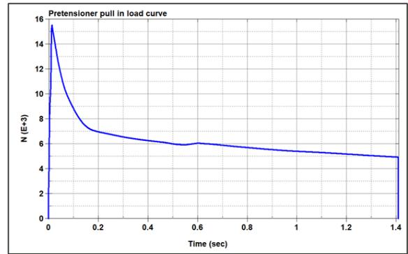
**Figure 8:** Pretensioner load curve
