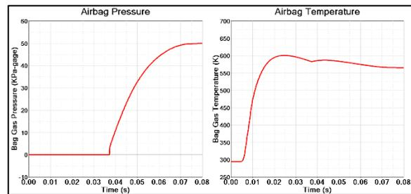
Figure 10: Airbag gas pressure and temperature
