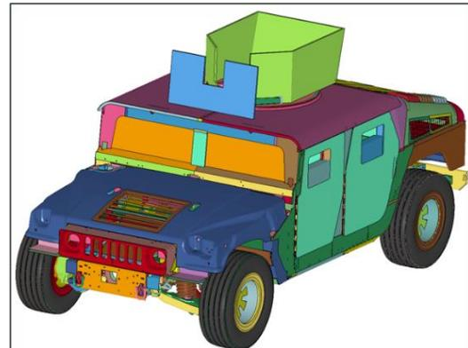
**Figure 18:** Integrated HMMWV model
