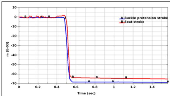
**Figure 33:** Buckle and seat pull in curves.
