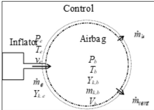
Figure 9: Airbag inflation process
