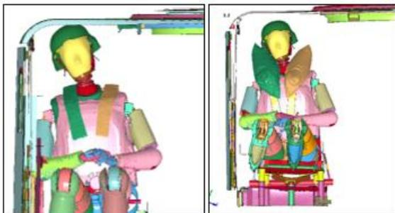
**Figure 32:** Passenger head with deployed neck bag
