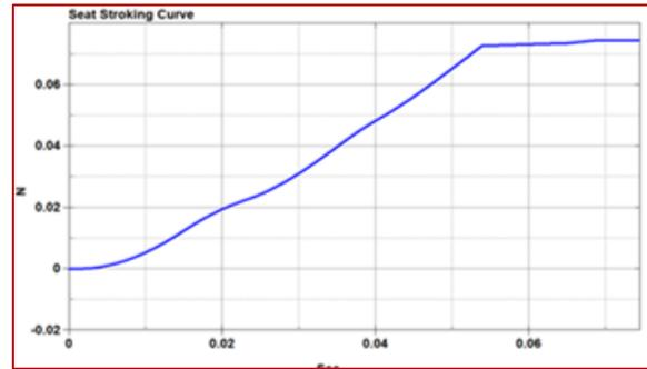
**Figure 13:** Pull down seat stroking load time history curve.
