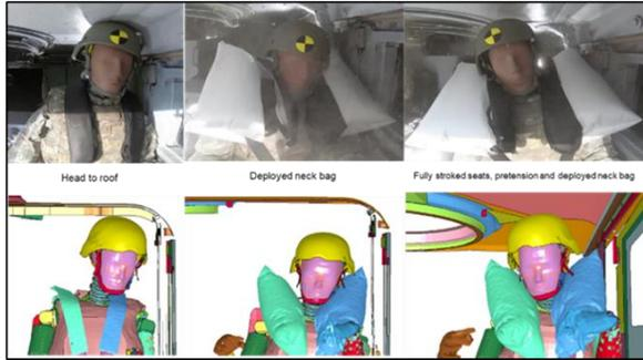
**Figure 31:** Deployed airbag and head-neck positions
