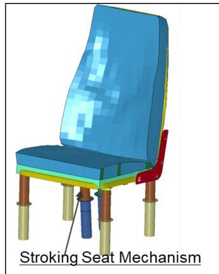
**Figure 14:** Pull down seat model.
