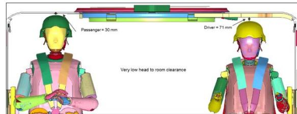
**Figure 17:** Head to roof clearance
