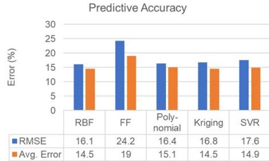
Figure 11 Predictive accuracy of various scalar surrogate model types for APS-CE endgame.
