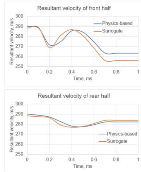
Figure 14 Velocity time history comparison from the threat break-up into two pieces
