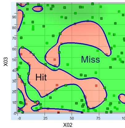
Figure 9 Explicit design space decomposition through classification technique showing regions of potential hits to the vehicle and misses (based on a given target swerve) plotted against two input variables.
