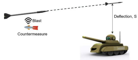
Figure 6 Deflection of a KE threat using APS hard-kill, also sometimes referred to as swerve.
