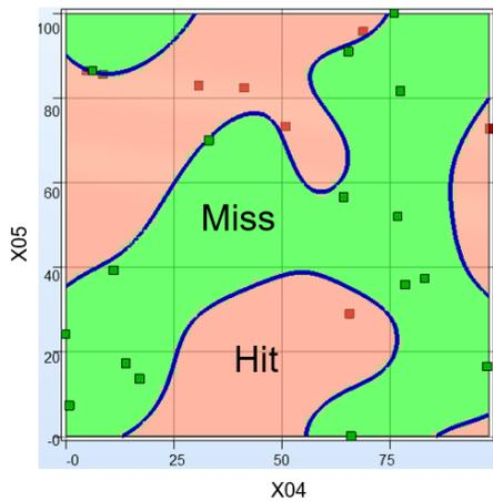
Figure 13 Explicit design space decomposition through classification technique showing regions of potential hits to the vehicle (APS failing to deflect or break up the threats) and misses (APS deflected and dismembered threats) plotted against two input variables.
