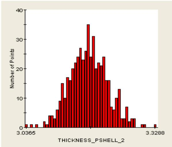
**Figure 14:** Thickness variation (mm).
