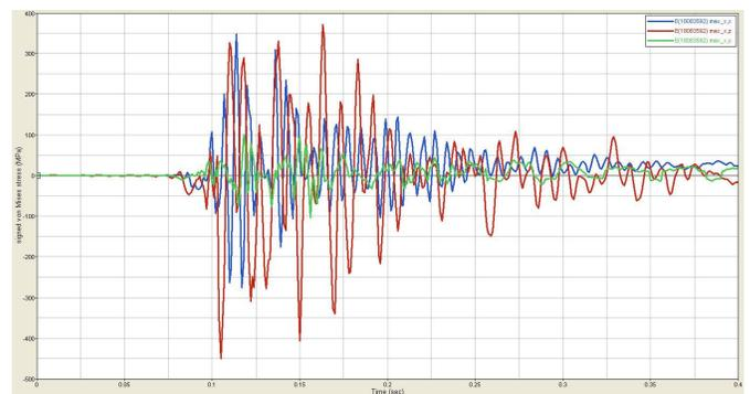
**Figure 9:** An example of transient stress response.
