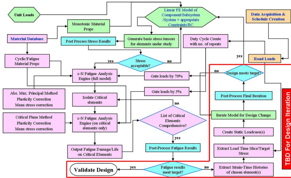
Figure 10: Fatigue life process.
