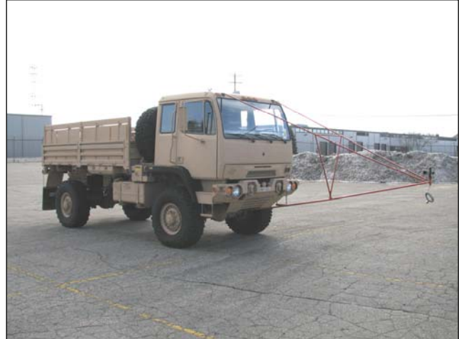
Figure 11: FMTV wind sensor installation
