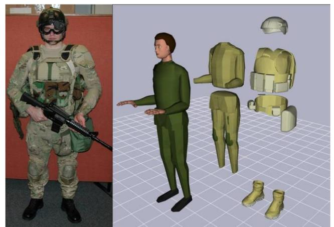
Figure 3: SME defined equipment and its distribution on a Soldier body relative to the digital model.
