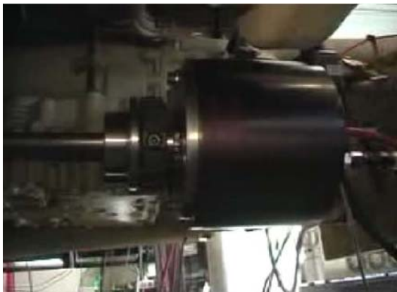
Figure 11: PMDC power system mounted in test vehicle
