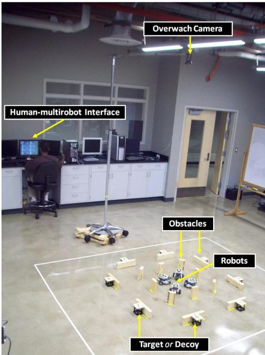
**Figure 1:** A group of semi-autonomous robots is controlled using the human-multirobot interface.
