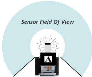
**Figure 3:** A marker is attached on the top of a NXT robot. The marker is detected by AR software to measure a robot position and to generate virtual images to merge with a robot in real time. An infrared sensor with a 240 degree view is attached on the NXT robot to search and detect infrared beacons.
