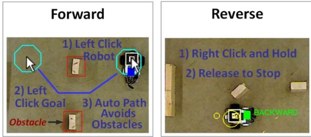
**Figure 6:** The path planning algorithm allows the multiple robots to traverse to the target location with obstacle avoidance and shortest path.
