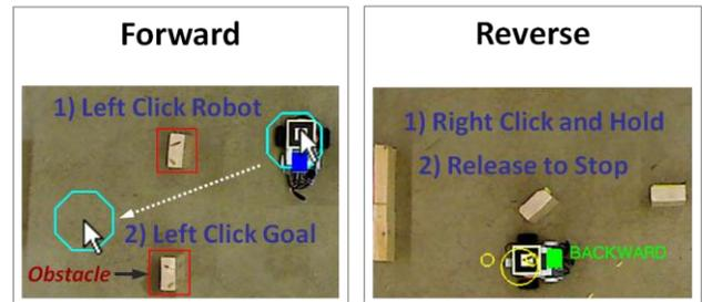
**Figure 5:** Point-and-Go is a high level instruction that allows an operator to control multiple semi-autonomous robots simultaneously.
