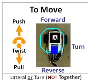
**Figure 7:** Push / pull the joystick to move the robot. Twist the joystick to turn the robot.
