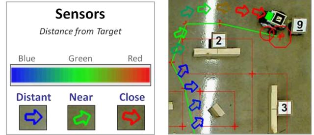
**Figure 8:** The robots detect infrared signals and drop “pebbles” when in motion. Arrows indicate direction and distance to a source.
