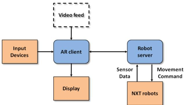
**Figure 4:** AR client programs share robot state information and display the synthesized view. Robot server programs read robot sensor data and send movement commands.
