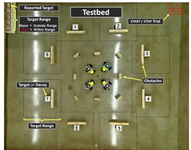
**Figure 2:** The human-multirobot interface is a top-down view from the stationary camera. We assumed that the top-down view could be taken from a manned or unmanned aerial vehicle.
