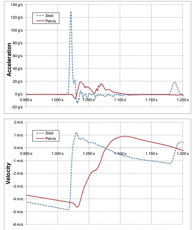
**Figure 2. Acceleration and velocity of the sled and the ATD during a drop test.**
