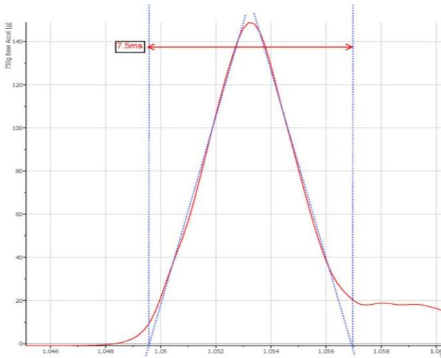
**Figure 5. A measure of pulse wide for drop tower impulse testing.**
