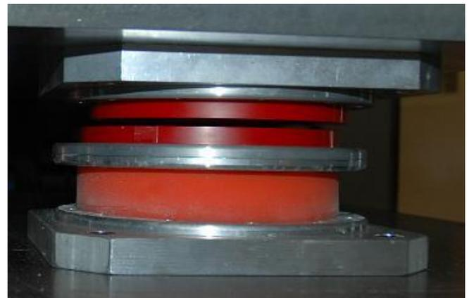
**Figure 4. Elastomer programmer used for pulse shaping on the GDLS drop tower.**
