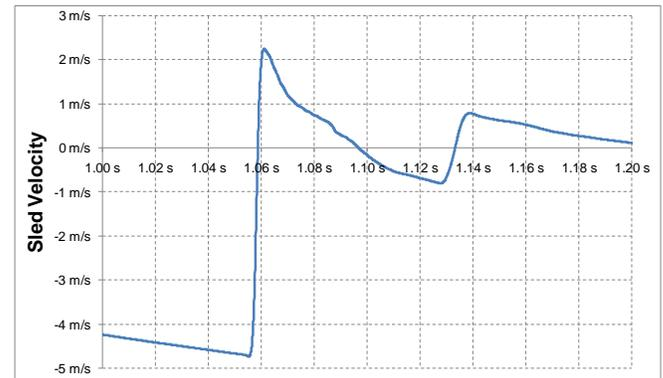
**Figure 3. Velocity trace from the sled of a drop tower showing anomalies.**
