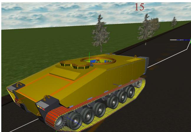
**Figure 22.** Snapshot of the motion of the tracked vehicle with a continuous belt track modeled using thick beam elements.
