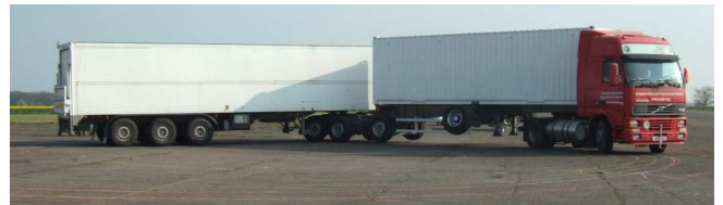
Figure 4: The Cambridge Vehicle Dynamics Consortium’s test vehicle, configured as ‘B-double’, fitted with active rear steering hardware on the two trailer axle groups
