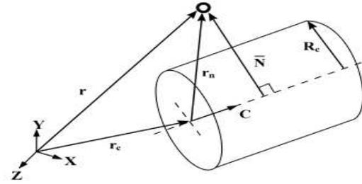
**Figure 3:** Geometry of contact between rigid cylinder and the  $C^0/C^1$  chain
