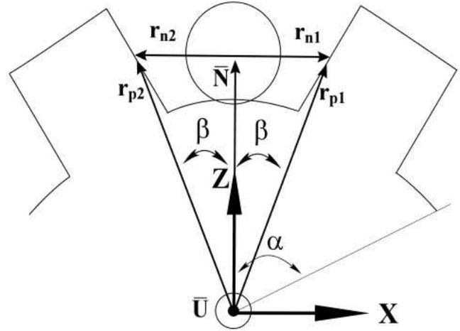
Figure 2: Geometry of contact between rigid sprocket teeth and the  $C^0/C^1$  chain
