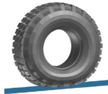
Figure 5: FEA Off-road tire model under 55 kN load and 0.6 MPa inflation pressure.
