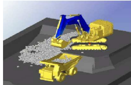
Fig. 1 . Hydraulic Excavator Bucket Loading – Dumping Operation (Granular Material) using Rocks3D TD
