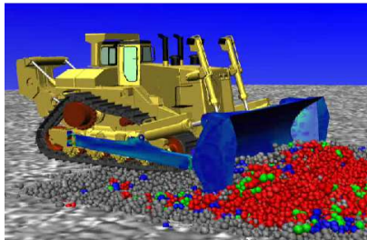
Fig. 4. D11 Track –Type Tractor Dozing Operation in Coehsive Soil using Rocks3D TD
