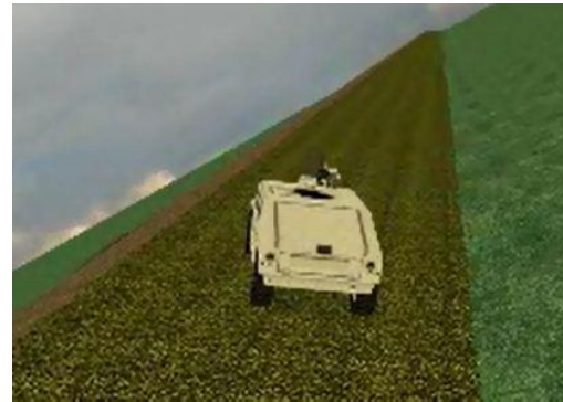
Figure 22: Vehicle slide over a dry sand slope @0.6 rad
