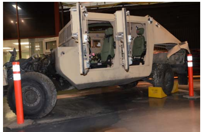
Figure 13: Fully integrated vehicle after underbody blast test.
