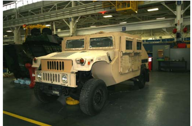
Figure 12: Fully integrated blast cab on existing HMMWV production chassis.
