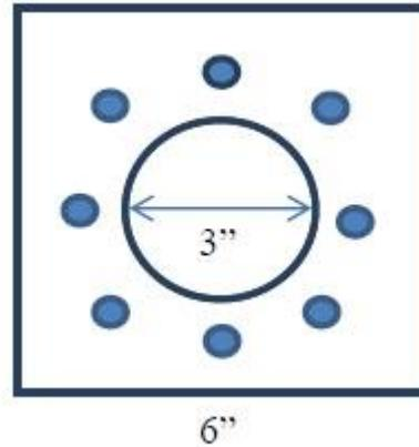
Figure 2. A drawing of a 3in diameter test specimen.
