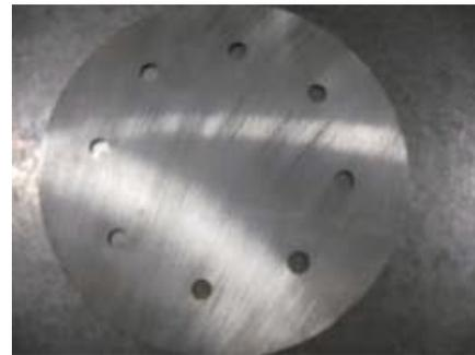
Figure 3. Photo of a 3in diameter AL 2139-T8 test specimen.
