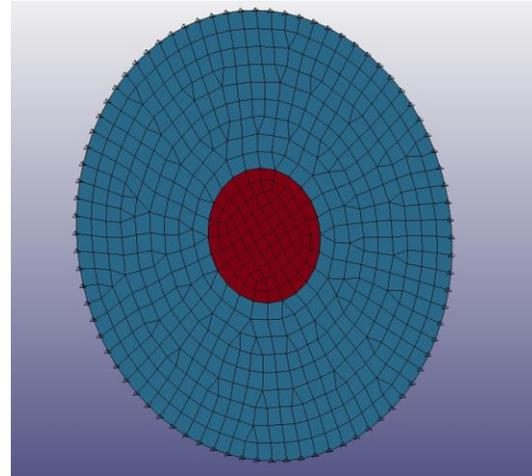
Figure 5. Shock tube finite element model.
