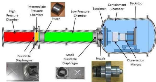
Figure 1. Schematic of a shock-tube with shock-tube components.
