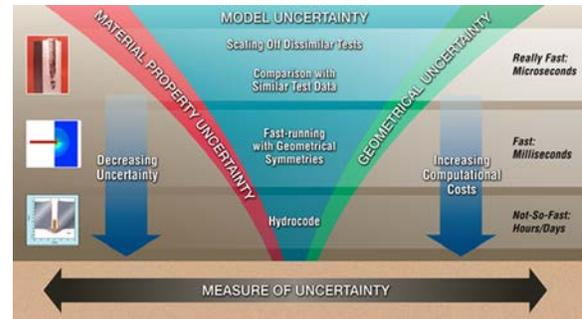
**Figure 2:** Multi-fidelity modeling (tiers of models) vs. analysis time and uncertainty – both the blast and ballistics survivability tools had low tier models that ran extremely fast, and high-tier models that had very high fidelity.
