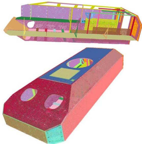
**Figure 4:** Images during the automatic production of a mesh for a ground vehicle; the meshing of this vehicle including interior structural members took 4 to 5 minutes on a PC.
