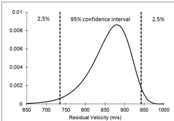
**Figure 8:** Computation of 95% bounds for the residual velocity from the Walker-Anderson model based on historical known variations in inputs to material properties and geometry.
