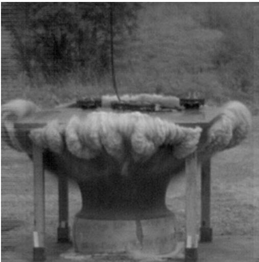
**Figure 10:** Stills from high speed video of an experiment to measure the loads produced by a buried charge.
