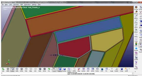
**Figure 6:** Images of a meshed conceptual hull showing the automatically produced heat affected zones (HAZs) surrounding all the automatically produced welds.
