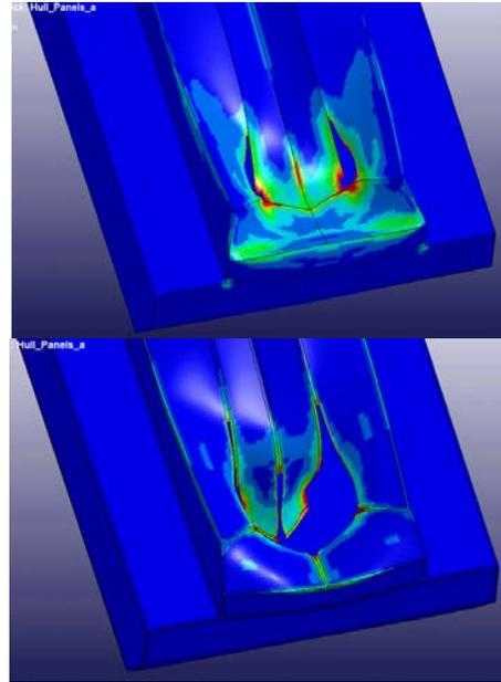
**Figure 7:** Images of a blast computation on a conceptual hull without an HAZ (above) and with an HAZ (below), showing the importance of including the HAZ. The HAZs and the welds in these examples were automatically produced by the tools developed for this program.
