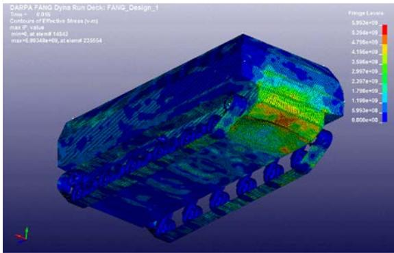
**Figure 12:** Blast loading by a buried explosive of a tracked infantry fighting vehicle, where the analysis and frame from a movie were automatically produced using the new software tools.
