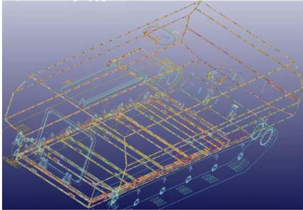
**Figure 5:** Image of automatically produced welds for a vehicle mesh.
