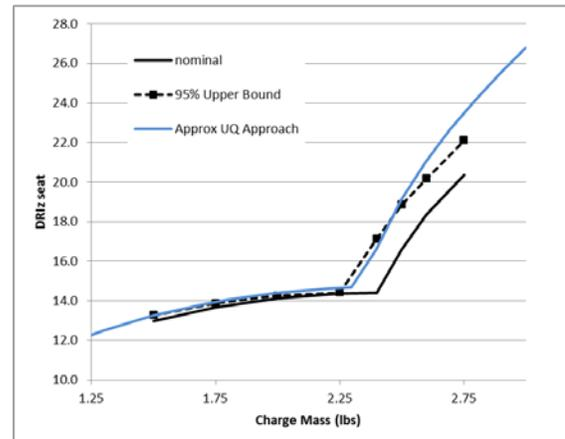
**Figure 9:** Computations with the Walker-Anderson model (upper, solid line) showing comparison to test data and then a second set of computations using adjusted input values (broken line) to produce a 95% bounding model; similar bounding results for spinal injury during blast (lower).
