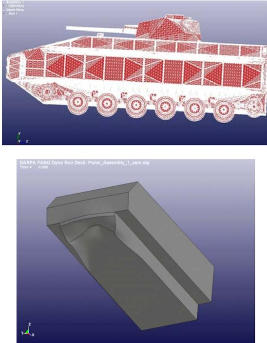
**Figure 3:** Motion from a Tier 1 blast under a front tread of a detailed design (upper) and a Tier 2/3 blast near the front of the conceptual hull (lower). The analysis of the first takes seconds and of the second is on the order of an hour.
