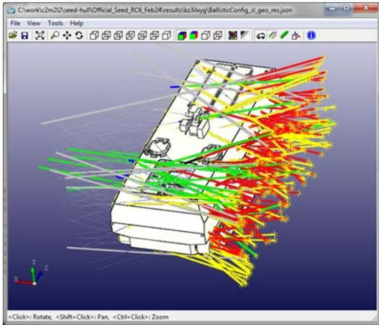
**Figure 1:** Screen image from the Shotline Viewer showing color-coded shot lines through the vehicle.
