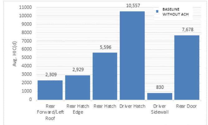
Figure 15: Vehicle B Baseline Head Impact Testing
