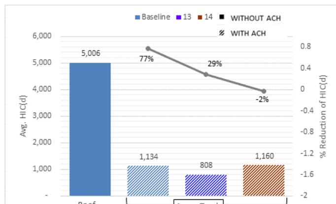
**Figure 25:** Ancra Track HIC(d) and Percent Reduction
