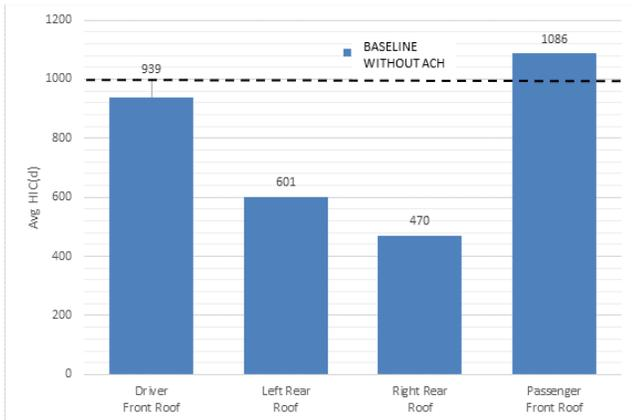
Figure 14: Vehicle A Roof Position Head Impact Testing
