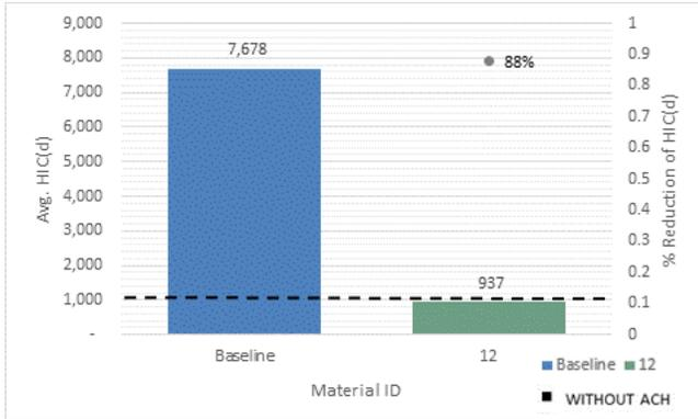
Figure 21: Rear Door HIC(d) and Percent Reduction
