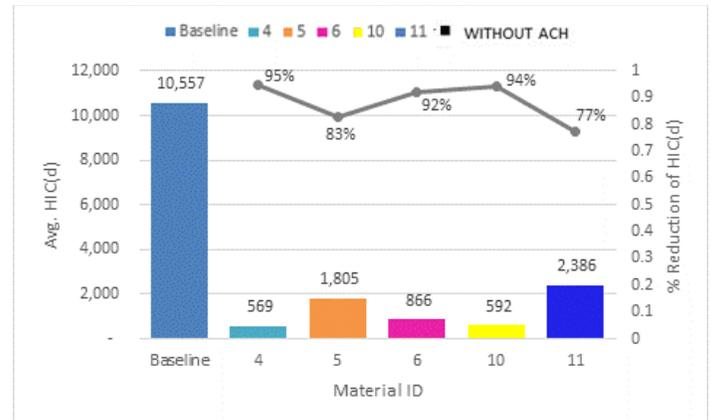
**Figure 19: Driver Hatch HIC(d) and Percent Reduction**
