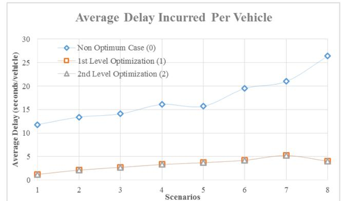
**Figure 4 – Plot of Average Delay Incurred Per Vehicle Under Different Cases and Scenarios**
