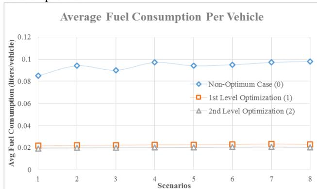
**Figure 3 - Plots of Average Fuel Consumption Per Vehicle Under Different Cases and Scenarios.**
