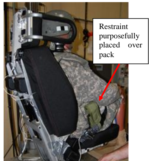
Figure 5: Rear Right Oblique View of ATD with Misplaced Restraints
