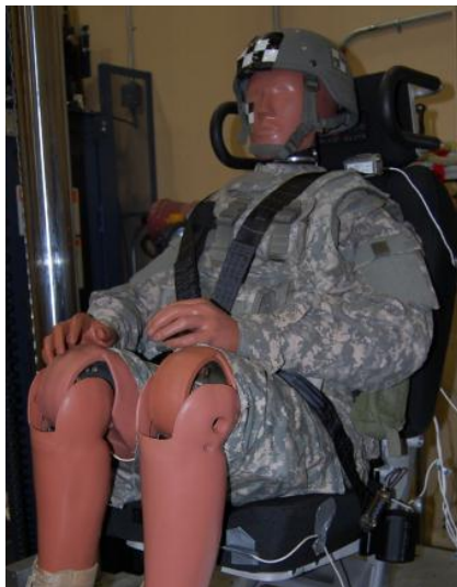
Figure 7: Front Left Oblique View of ATD with Misplaced Restraints
