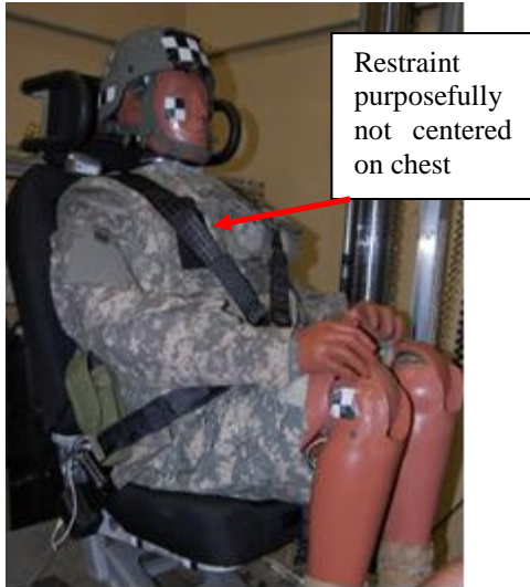
Figure 6: Front Right Oblique View of ATD with Misplaced Restraints
