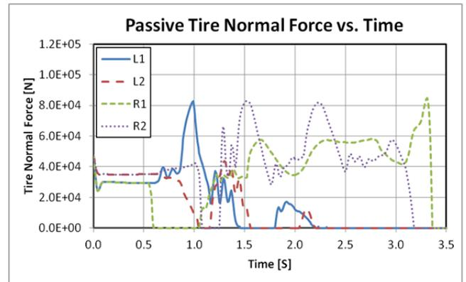
Figure 10 - Passive tire forces
