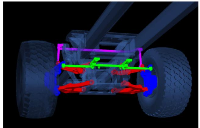
**Figure 5 - Modeled suspension system geometry**
