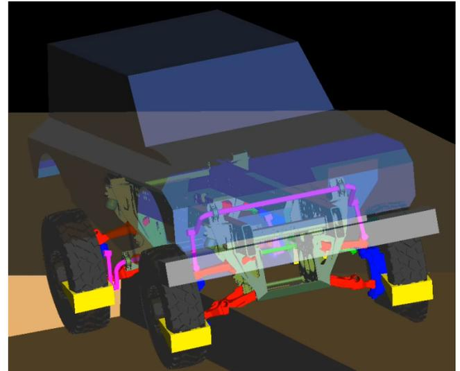
**Figure 18 - Frame-bottomed stuck state**
