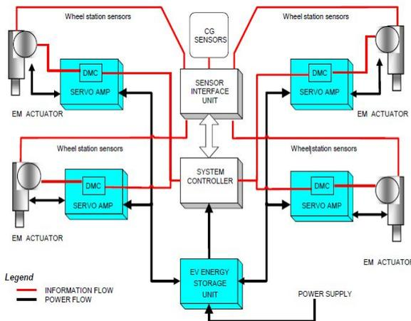
Figure 6 - EMS control architecture
