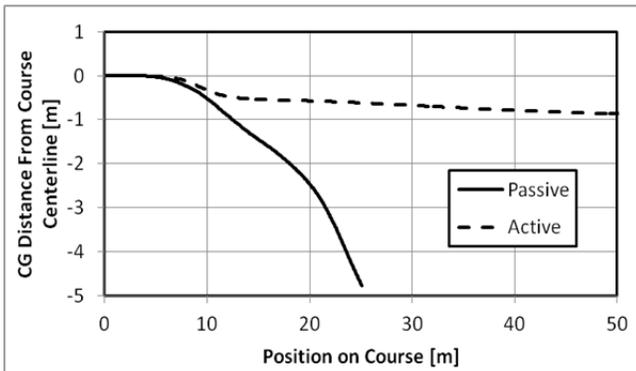
**Figure 14 - Vehicle path comparison**
