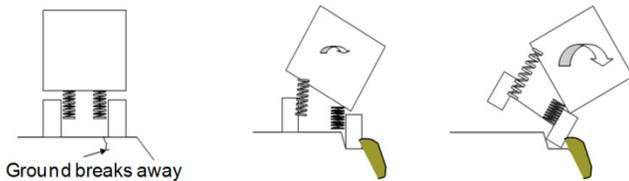
**Figure 1 - Vehicle rollover due to soil breakaway**
