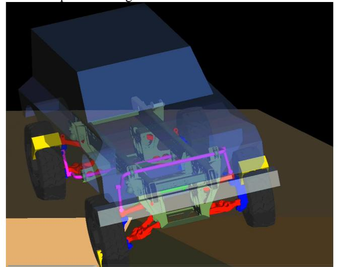
**Figure 16 - Stuck vehicle extraction, right front tire no longer in contact with terrain**
