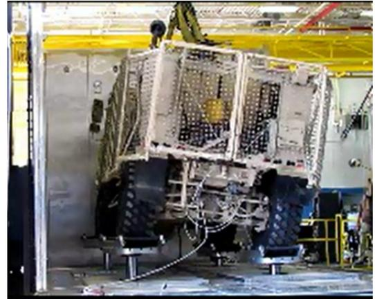
**Figure 2 - n-post Shaker simulating soil breakaway condition**
