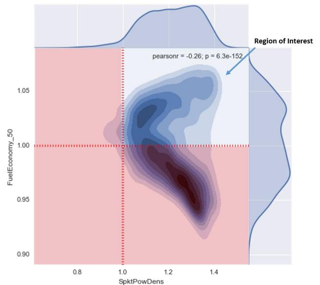
**Figure 5:** Joint Probability Distribution for Sprocket Power Density and Fuel Economy at 50 mph
