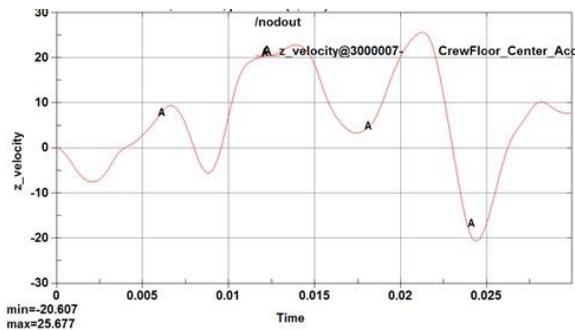
Figure 8: crew floor velocity result for simplified box model
