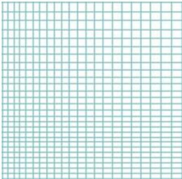
**Figure 1:** A structured mesh
