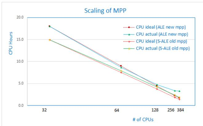
**Figure 12:** MPP scaling comparison between S-ALE and ALE with new MPP
