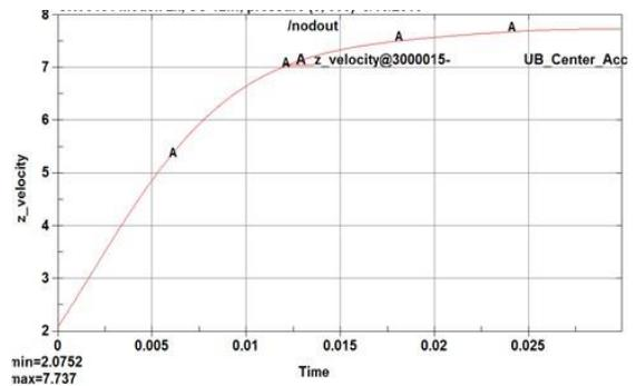
Figure 6: Underbody velocity result for simplified box model
