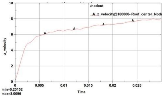
Figure 7: Roof velocity result for simplified box model
