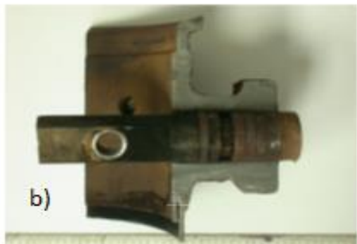
Figure 11: Dissected Butterfly Valve Shaft
