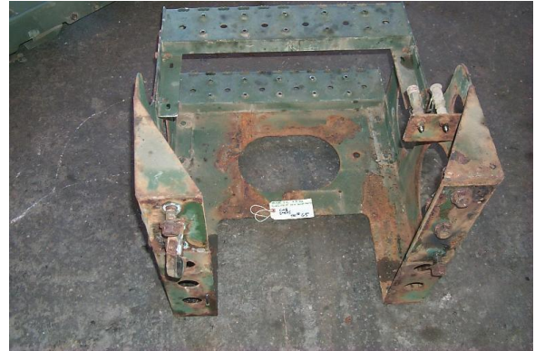
Figure 45: MTRV Mounting Ladder Coating Deterioration during ACDRT
