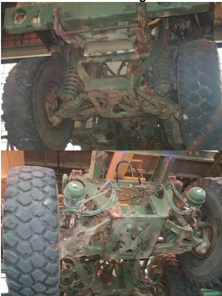
Figure 44: Underbody Suspension Coating Deterioration during ACDRT
