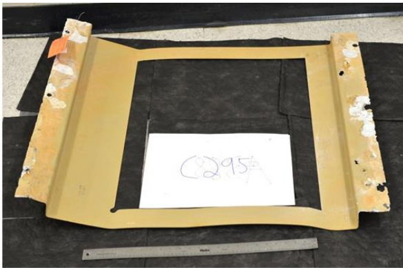
Figure 16: Aux. Trans. Cooler Shroud after ACDRT.
