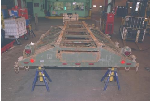
Figure 42: Coating Deterioration on the MTRV Truck Bed Frame during ACDRT
