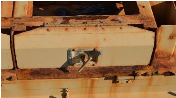
Figure 9: FMTV Stowage Door at the End of 22-year-Test
