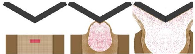
Figure 5. SPH Response Evolution for EMI 120-deg Plate Impact Simulation
