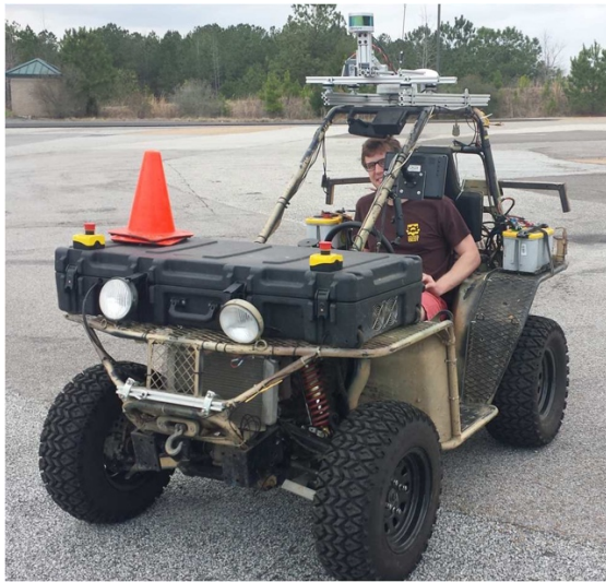
Figure 13: Prowler UGV with Velodyne VLP-16 scanner mounted to the roof.
