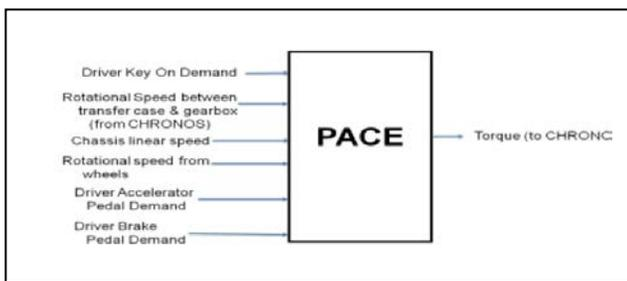
**Figure 3:** Illustration of inputs and output from the current version of PACE. Future versions will expand to accommodate additional inputs and outputs as needed [13].
