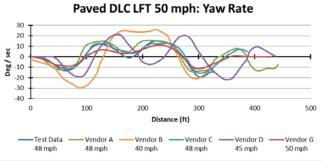
Figure 5: Double Lane Change Comparison to Test Data
