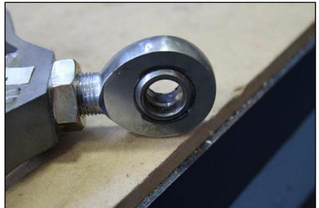
**Figure 31:** Post-test inspection of rod end in good condition.
