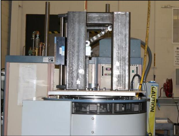
**Figure 8:** Electrodynamic shaker used to provide road vibration loads.
