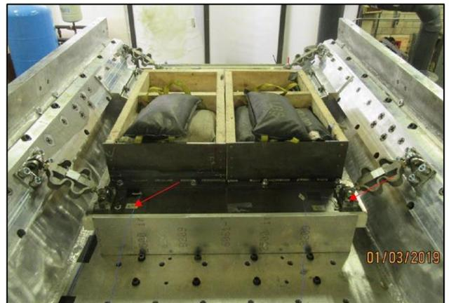
**Figure 28:** Test setup for road shock (crew configuration shown).
