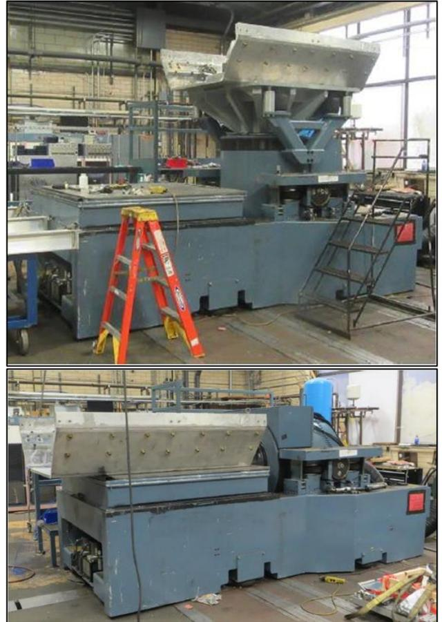
**Figure 27:** Electrodynamic shaker in vertical (top) and horizontal (bottom) configurations.
