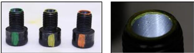
Figure 9: Hollow tensile screw design.
