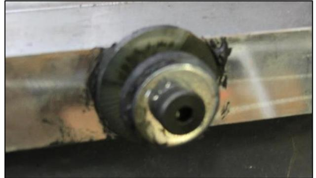
**Figure 29:** Post-test inspection of transverse panel bushing in good condition.
