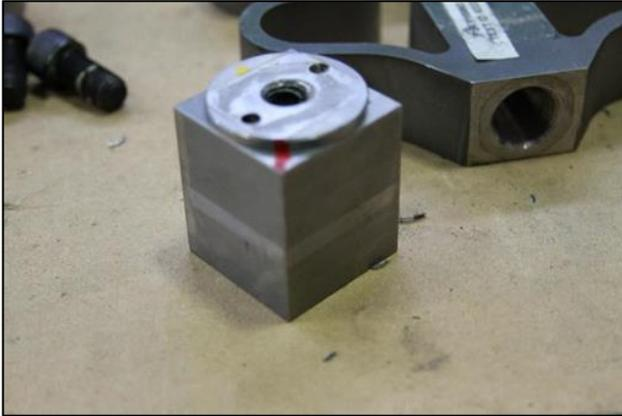
**Figure 32:** Post-test inspection of tensile screw assembly.
