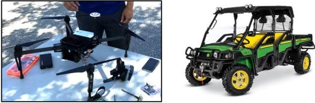
Figure 12: LEFT: DJI Matrice 100 Quadrotor UAV with large surface for mounting instrumentation. RIGHT: Instrumented John Deere Gator research vehicle
