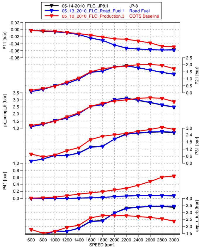
**Figure 10 - Effect of removing COTS Exhaust Aftertreatment System on Air Handling System**
