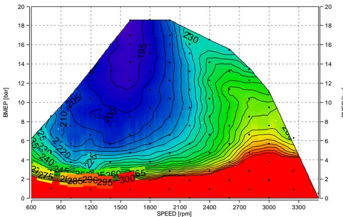
Figure 16 – Brake Specific Fuel Consumption on JP-8 (g/kW-hr)
