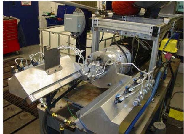
**Figure 24 - AVL Fuel System Durability Bench Rig**
