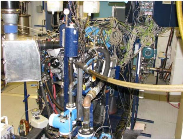
**Figure 8 - 6.7L Engine Installation in AVL Test Cell**
