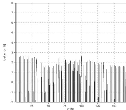
**Figure 22 - Engine Control Unit Fueling Error During NATO Cycle Test**
