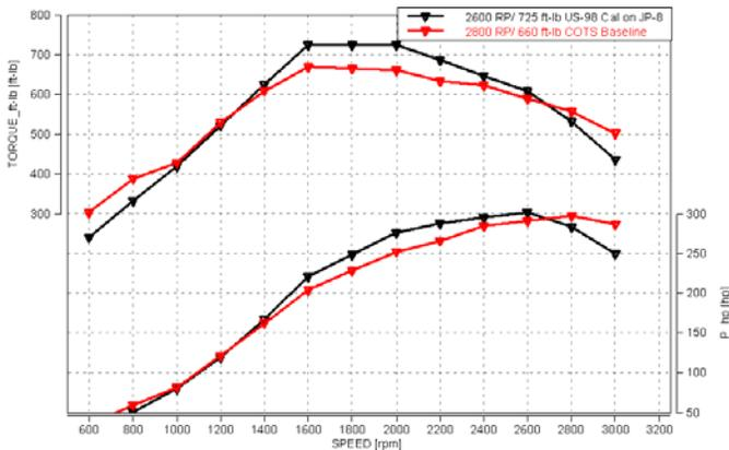
Figure 13 - Full load Torque and Power Curves
