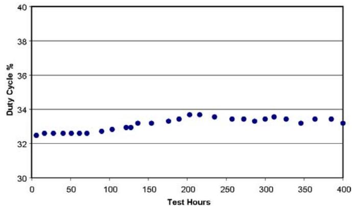
**Figure 27 - Volume Control Valve Signal Throughout Fuel System Durability Test**
