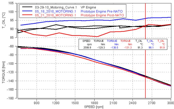
**Figure 23 – Engine Motoring Torque Before and After 50 Hour NATO Cycle Durability Testing**
