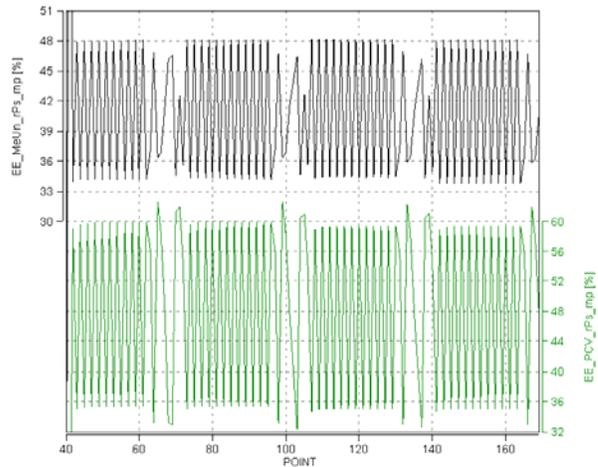
**Figure 21 – Fuel System Pressure and Volume Control Commands During NATO Cycle Test**
