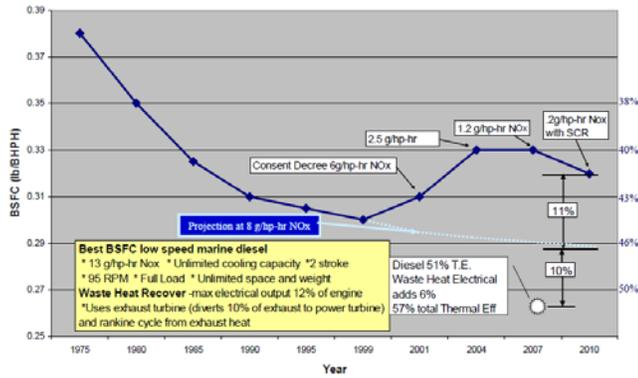
**Figure 6 – Impact of Emission Regulations on Heavy-Duty Engine Minimum BSFC Levels [2]**
