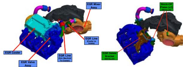
**Figure 9 - Removal of the COTS EGR system**
