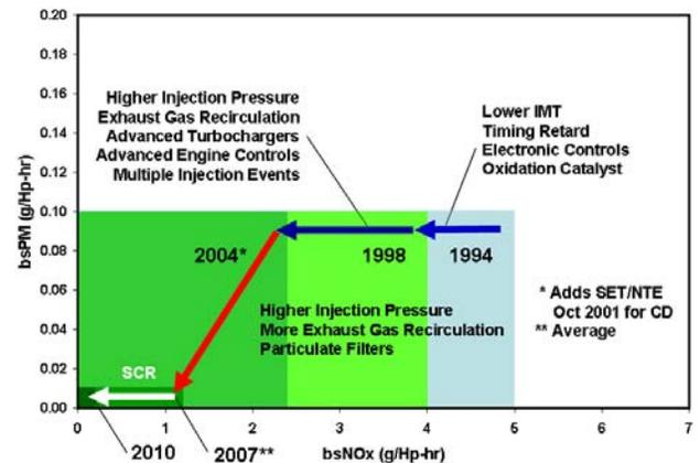
**Figure 2 - Emission Control Technology Solutions**
