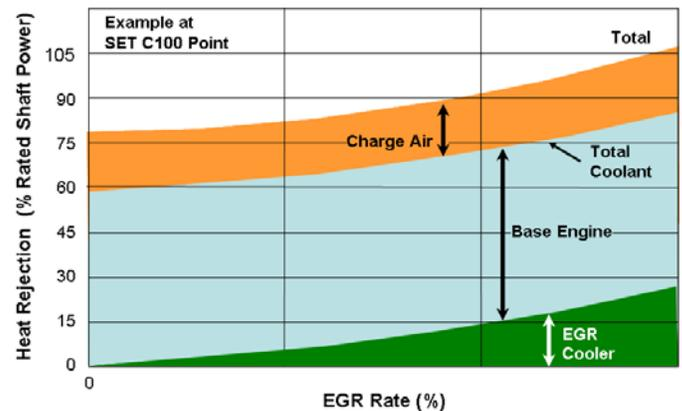
Figure 4 - Impact of EGR on System Heat Rejection
