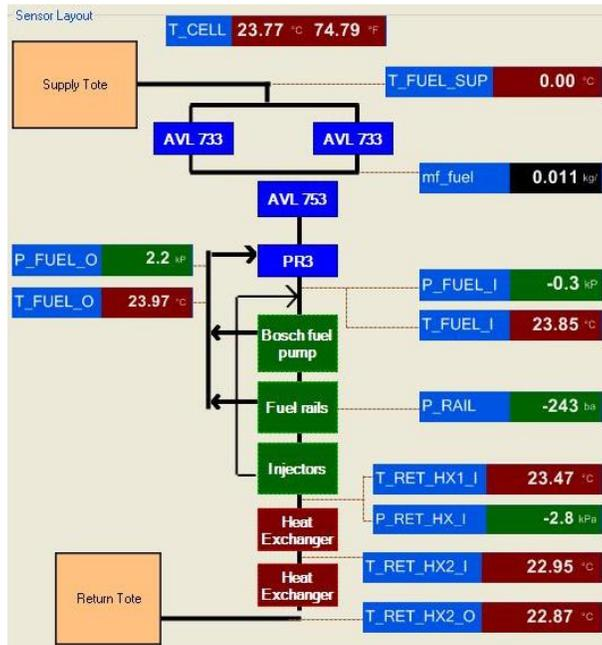
**Figure 25 - AVL Fuel System Bench Schematic**
