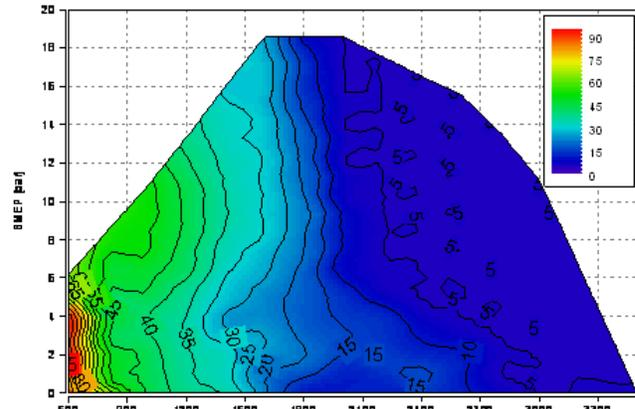
**Figure 11 - VGT Commanded Position, Final Calibration (5=fully open)**
