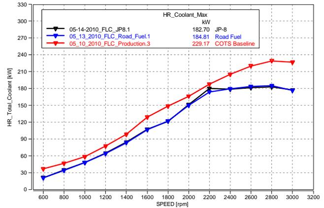
Figure 14 - 20% Reduction in Total Heat Rejection
