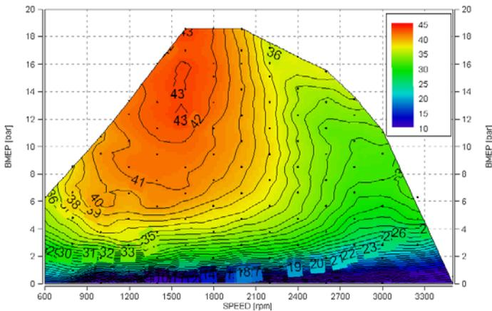
Figure 15 – Brake Thermal Efficiency on JP-8
