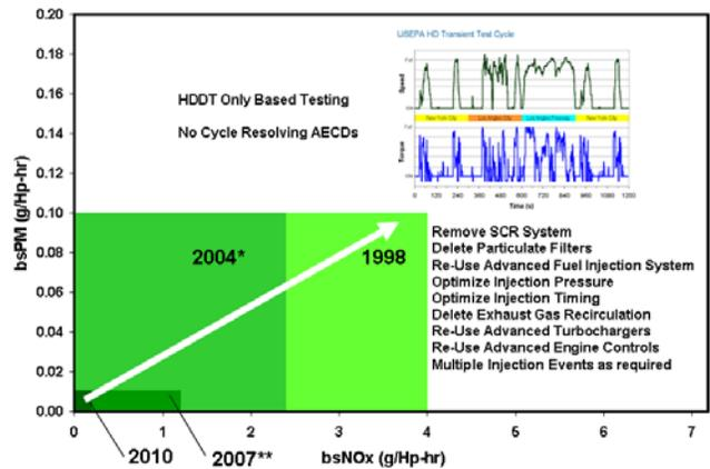
**Figure 7 - Technology path for defense applications using JP-8**
