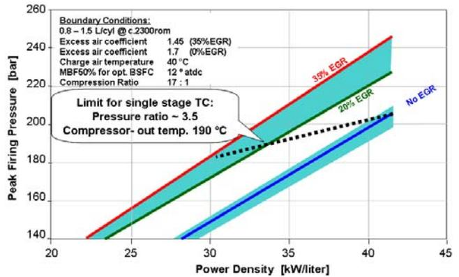
Figure 3 - Impact of EGR on Peak Firing Pressure
