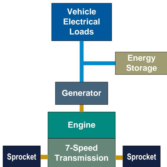
**Figure 8. Mechanical Drive.** A 7-Speed transmission is used to represent mechanical drive attainable performance.
