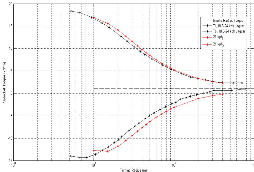
**Figure 6. Sprocket Torque vs Turning Radius.** The ISM terramechanics model is validated against Jaguar tracked vehicle experimental data.
