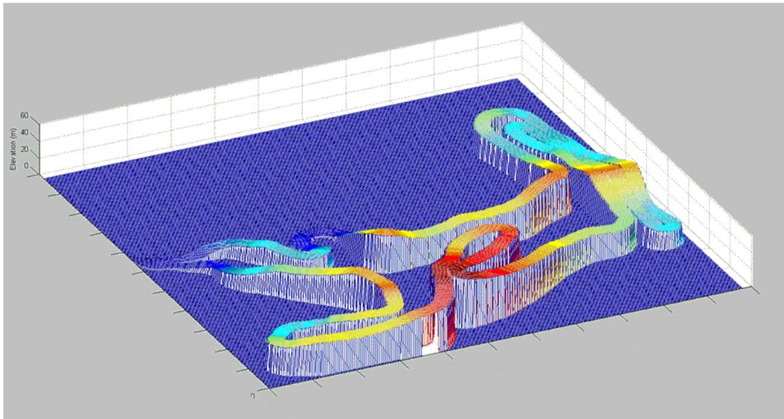
**Figure 5. Three-dimensional Churchville B Cross Country Course Profile.** Selected segments of this hilly profile with turns are used to represent portions of the total mission profile.
