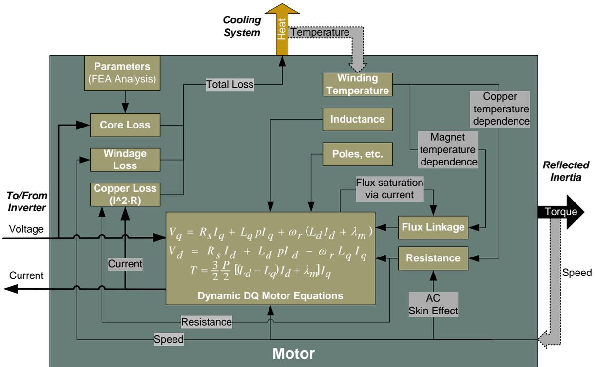
**Figure 3. Detailed Component Model Interaction.** The element models capture the multidomain interactions such as how the resulting component temperatures affect the component's performance characteristics to more accurately predict performance and losses.
