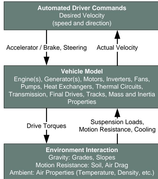
**Figure 1. Top Level Integrated System Model.** The generic block diagram for the vehicle provides great flexibility to how the vehicle interacts with a variety of driver commands and the environment in which the vehicle is operated.
