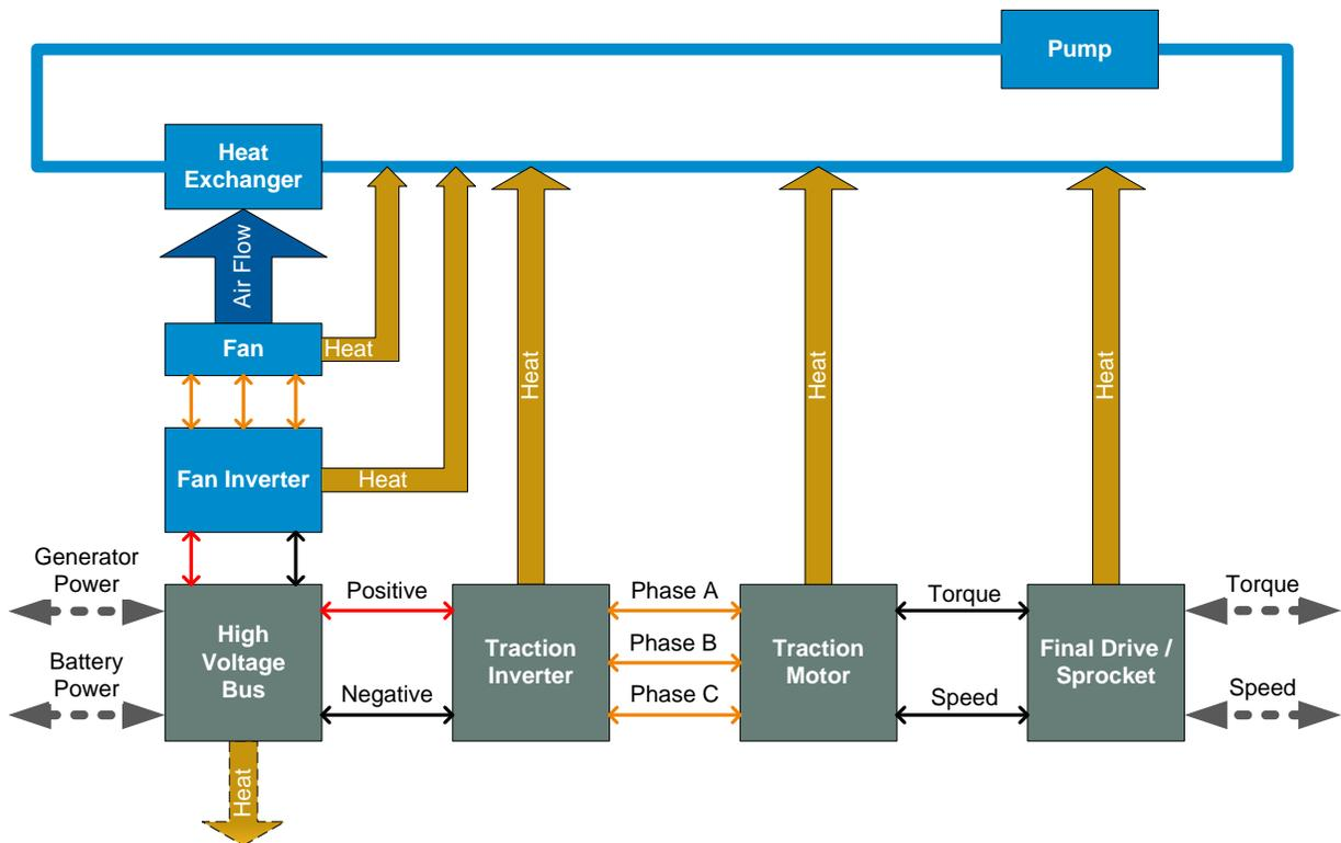
**Figure 2. Component Model Interaction.** The multidomain physics-based component models capture mechanical, electrical and thermal interaction using well-defined interfaces.
