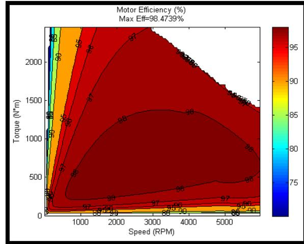
**Figure 7. Motor Efficiency Map.** Motor efficiency over the entire operating torque and speed range as a function of temperature is used to more accurately capture losses while operating over the duty cycle.
