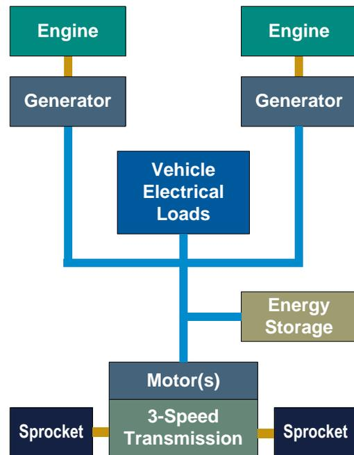
**Figure 9. Series Hybrid Electric Drive.** A 3-speed transmission with dual engines is used to represent series hybrid electric drive attainable performance.
