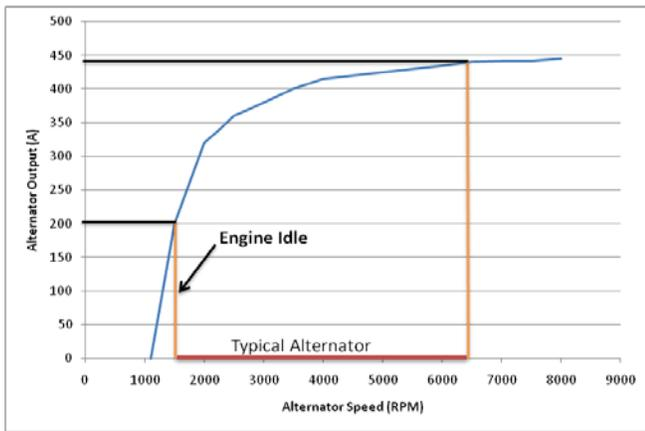
**Figure 2: Power curve for a typical 400 A alternator.**
