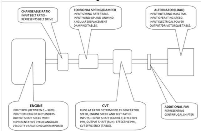
**Figure 5: System dynamic model for torque pulse simulation.**
