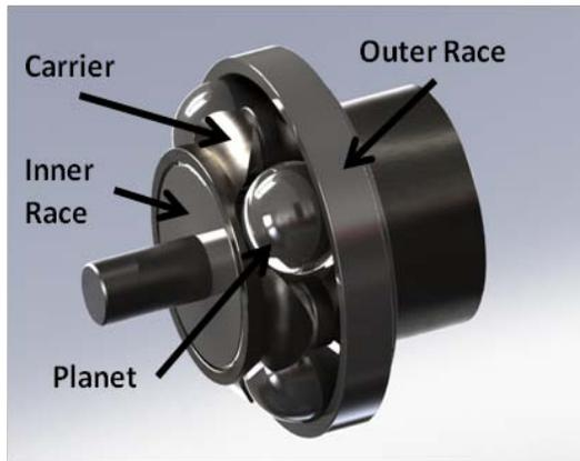
**Figure 4: Key CVT components.**
