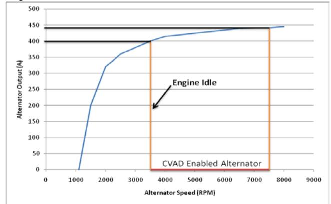
**Figure 3: Power curve for a CVAD-enabled 400 A alternator.**
