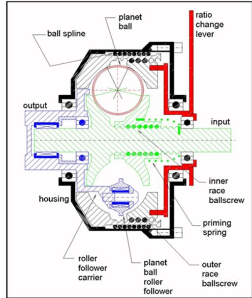
**Figure 6: Cross section of Orbital Traction's CVT.**
