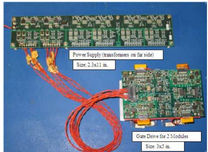
**Figure 8: Prototype Gate Drive and Power Supply Hardware for Thermal Evaluation**
