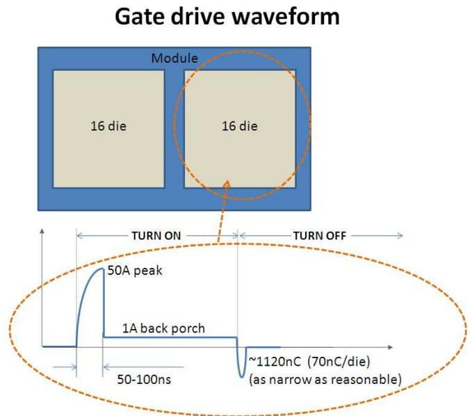
Figure 5: Module Switching Characteristics
