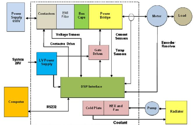
Figure 2: Traction Motor Drive Block Diagram
