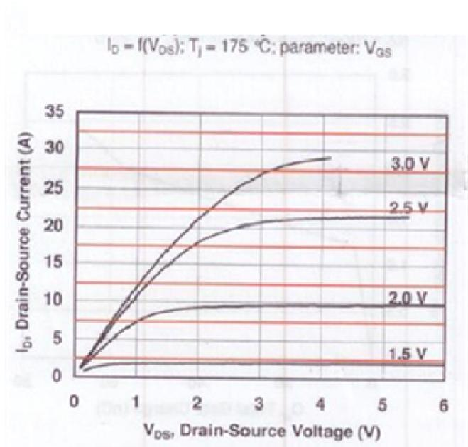
Figure 4: JFET Transconductance Characteristics
