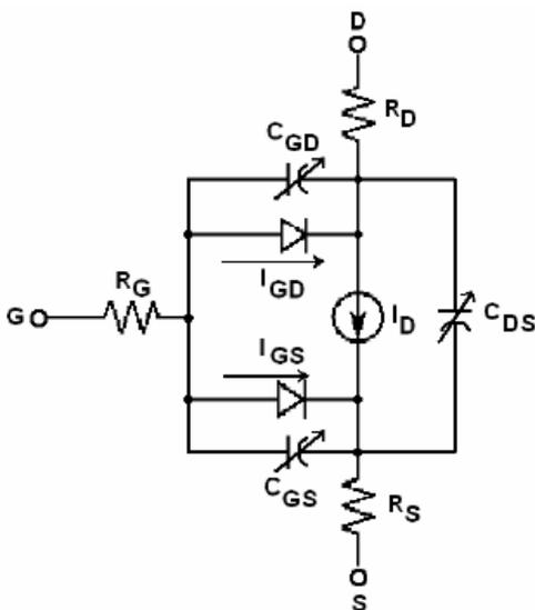
Figure 3: JFET Equivalent Circuit
