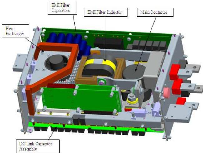
**Figure 14: Motor Drive Package, Internal, Bottom View**
