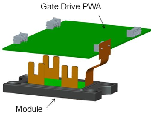
**Figure 6: Gate Drive and Module Arrangement**
