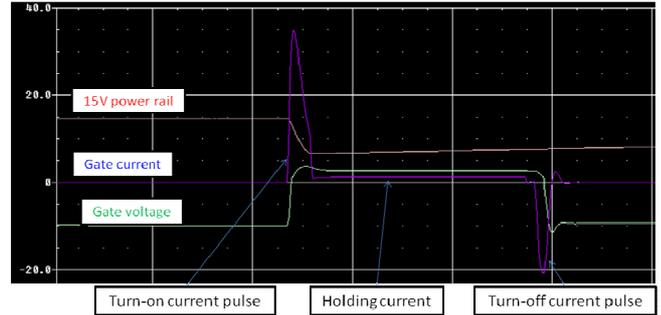
**Figure 7: Simulated Gate Drive Circuit Waveforms**
