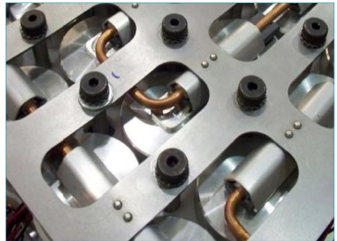
Figure 2. Detail photograph of an ultracapacitor array utilizing two-phase VDF cooling system concept for a heavy off-road vehicle with HEV powertrain.
