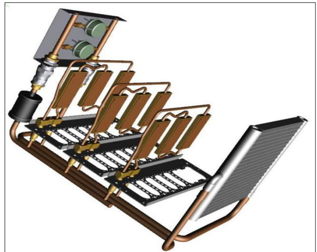
Figure 1: Conceptual layout of a modular VDF cooling system for a military ground tactical vehicle HEV powertrain inverter. Note that each cold plate module consists of three VDF liquid cold plates in series, to mount three standard IGBT modules for this prototype drive.
