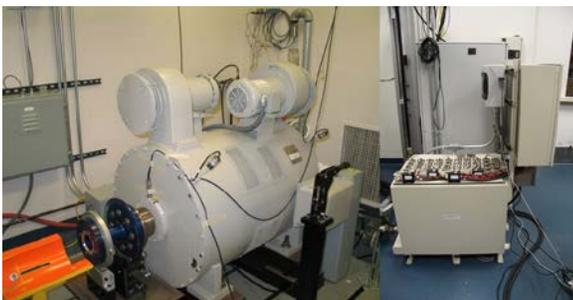
**Figure 3:** Dynamometer and Programmable Resistive Load bank
