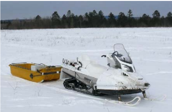
Figure 1: Loki Prototype with optional modular genset / cargo trailer sled attached
