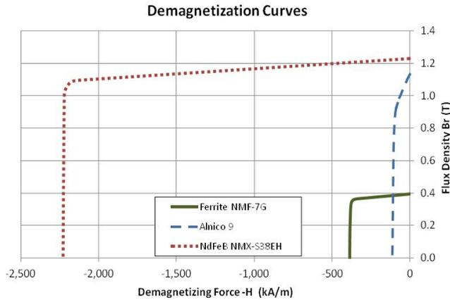
**Figure 5: Example demagnetization curves for PM materials at 20° C.**
