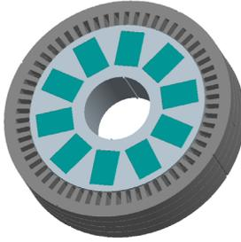
**Figure 6: Example Spoke IPM Structure.**
