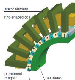
**Figure 7: Basic TFPM Structure.**
