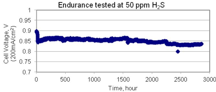
**Figure 4: Demonstration of the performance of a SOFC cell and membrane assembly operating with 50ppm H<sub>2</sub>S for 3,000hrs at approximately 200mA/cm<sup>2</sup>.**
