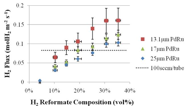
**Figure 3: Hydrogen permeable palladium membrane flux results for membranes with varied thicknesses.**
