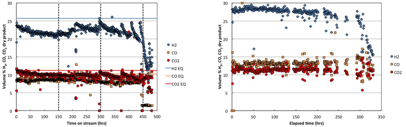
**Figure 2: Endurance reforming results for Rh-based Ceria catalyst, tested with 300ppmwS JP-8. Results for endurance operation (right) and cyclic operation (left) are shown.**
