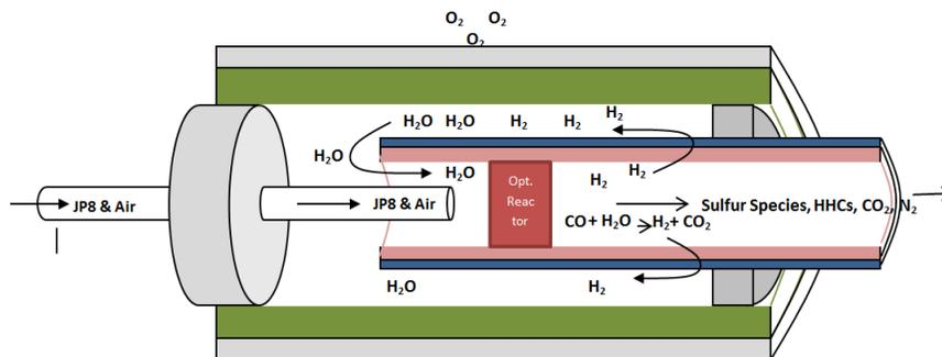
Figure 1: Schematic of the membrane-based JP-8 fueled SOFC cell design.
