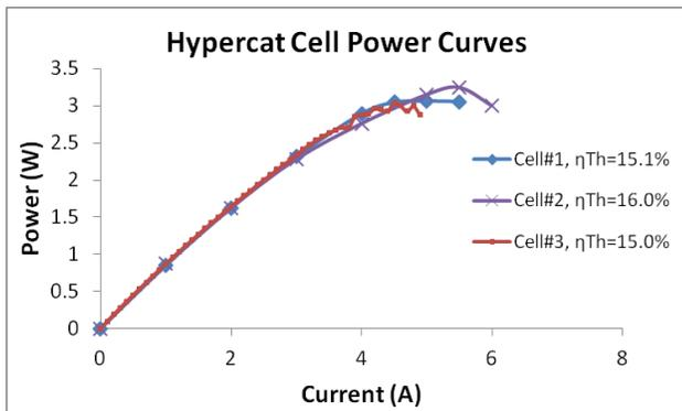
**Figure 5: Single cell (SOFC tube and membrane bundle) power curve operating utilizing JP-8 reformat (approximately 40ppmv H<sub>2</sub>S).**
