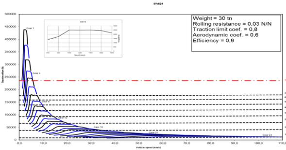
**Figure 7. 24- speed traction curves and ratios**
