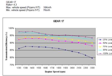
Figure 2.1. SG850 Efficiency Gear 17
