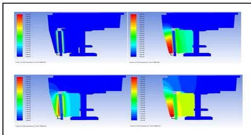
**Figure 9. Clutch thermal analysis results**
