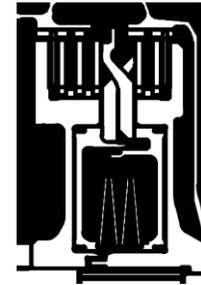
**Figure 10. Two clutches with single Chamber**
