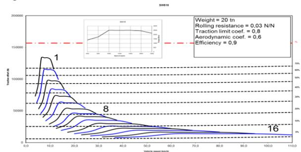
Figure 6. 16-speed traction curves and ratios
