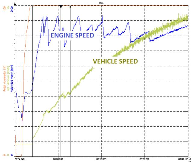
Figure 12. SG850 transmission acceleration
