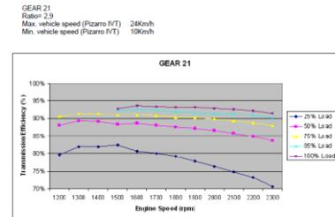
Figure 2.2. SG850 Efficiency Gear 21
