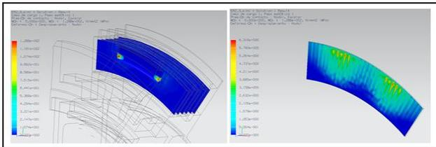
**Figure 8. Clutch pressure distribution calculation results**
