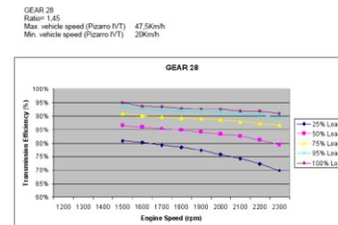
Figure 2.4 SG850 Efficiency Gear 28
