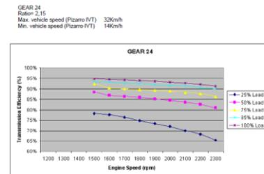
Figure 2.3 SG850 Efficiency Gear 24
