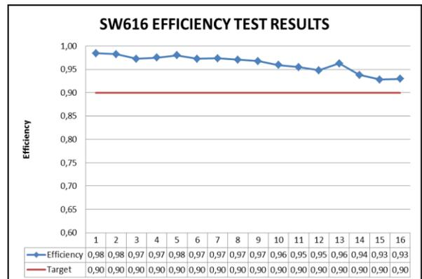
Figure 14.1. SW 616 Efficiency
