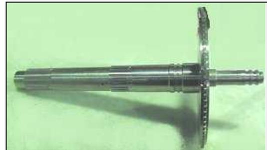
**Figure 11. SW616 and SW 624 central shaft**
