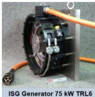
Figure 3: 75kW ISG System for Light Military Vehicle Applications
