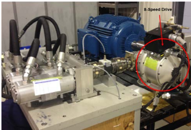
Figure 7 – Efficient PTO Fan Drive Testing at KTR
