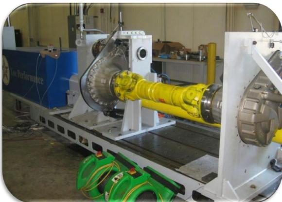
**Figure 4: Loc Final Drive Dynamometer**
