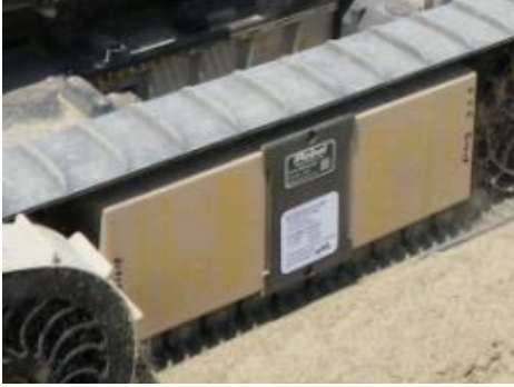
Figure 6. Situation of embedded BB-2590 batteries. (Yellow boxes between wheels)
