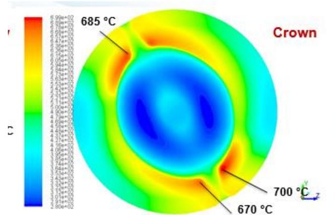
**Figure 7. Predicted piston crown temperature on the hot side of the inner piston (commercial SCOPE piston).**
