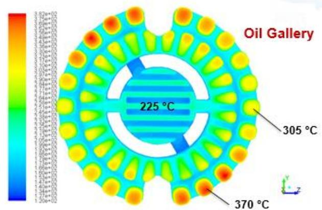
**Figure 8. Predicted back side piston temperatures of the inner piston (commercial SCOPE piston)**
