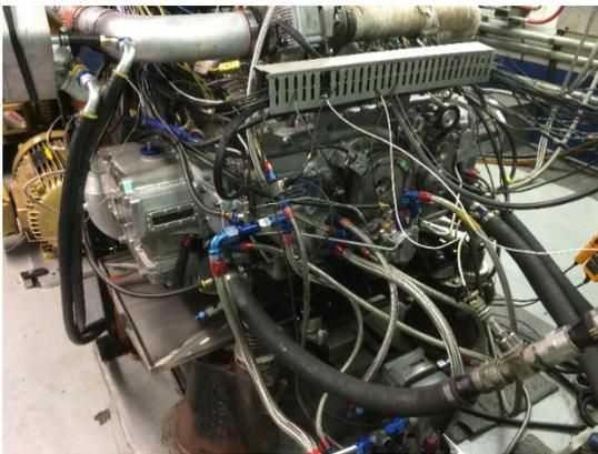
**Figure 4. Fully instrumented SCOPE engine used for determination of the heat rejection to power ratio.**
