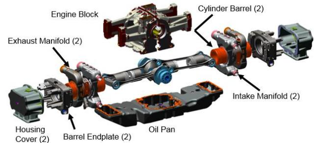
**Figure 3. Exploded view of the commercial version of the SCOPE configuration (outer core engine parts).**
