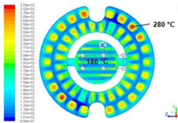
Figure 10. Predicted back side piston temperatures of the inner piston with a ceramic insert added (militarized SCOPE piston).
