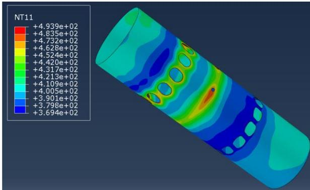
**Figure 5. Predicted temperature distribution of barrel surface temperature for the commercial SCOPE engine.**
