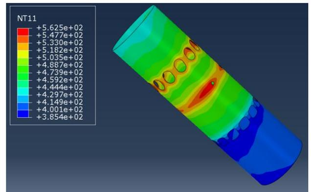
**Figure 6. Predicted temperature distribution of barrel surface temperature for the military SCOPE engine.**
