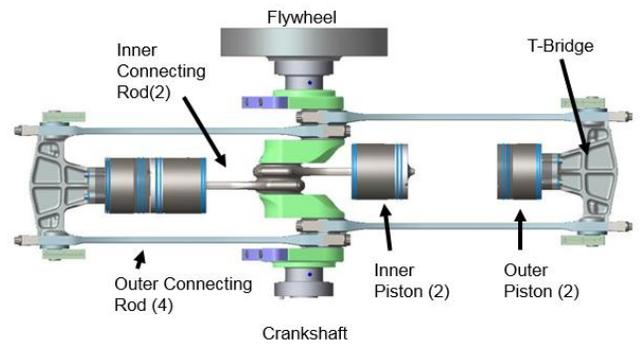
**Figure 2. Exploded view of the SCOPE engine (powertrain components).**
