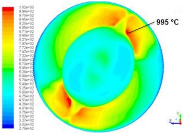
Figure 9. Predicted piston crown temperature on the hot side of the inner piston with a ceramic insert added (militarized SCOPE piston).
