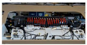
**Figure 8:** QinetiQ E-X-Drive® installed the 'Hotbuck' SIL (Photo courtesy BAE Systems).
