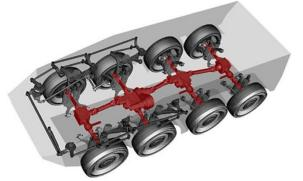
**Figure 2:** Boxer Multirole Armoured Vehicle (MRAV) (driveline highlighted in red). Photo courtesy UK Ministry of Defence (MOD).
