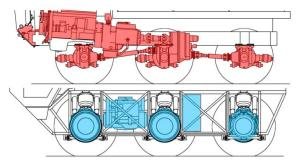
**Figure 3:** QinetiQ 6x6 powertrain comparison – conventional (red) vs. hybrid (blue).
