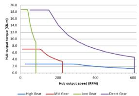
**Figure 10:** Hub drive torque-speed map (with hypothetical single-ratio direct-drive motor for comparison).
