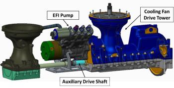
Figure 6 – Auxiliary Drive Arrangement
