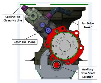
Figure 3 – EFI Pump Mount Orientation
