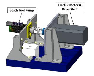
Figure 4 – EFI Pump Test Rig Concept
