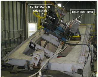
Figure 5 – EFI Pump Tilt Test
