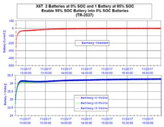
**Figure 5:** Parallel connection testing of fully charged Xcelion<sup>®</sup> 6T-Energy with two fully discharged batteries. Battery current displayed in Amps.
