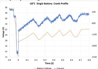
Figure 4: Vehicle cranking supported by a single Xcelion<sup>®</sup> 6T-Energy battery at -18°C without preheating
