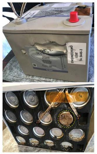
**Figure 7:** Abuse testing results of the Xcelion 6T Battery – yellow circle indicates abused/overheated cell
