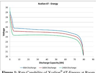
Figure 1: Rate Capability of Xcelion<sup>®</sup> 6T-Energy at Room Temperature
