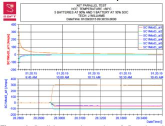
**Figure 6:** Parallel connection testing of five charged Xcelion 6T<sup>®</sup> batteries with one discharge battery
