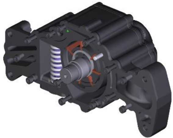
Figure 4: CAD Model of Pump Showing Internal Components
